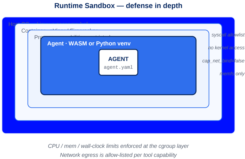
Figure 5.1 — Four nested isolation layers. The agent has the fewest capabilities; the host OS has the most.
